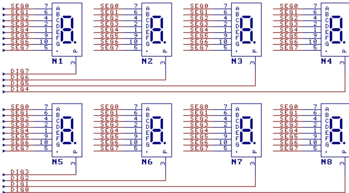
CH452 can drive 8 common cathode LED Nixie tubes dynamically. After the pins on the same segments of all LED Nixie tubes are connected in parallel (segments A-G and decimal point), they are connected with the segment drive pins SEG0-SEG7 of CH452 through a series current limiting resistors R1 (or R12). The cathodes of each LED Nixie tube are driven by the pins DIG0~DIG7 of CH452 respectively.
