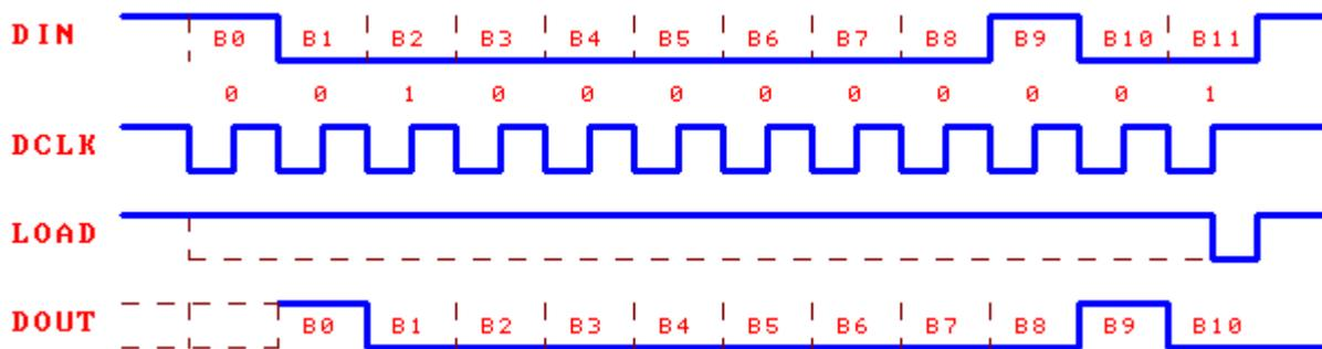
The figure above is a waveform diagram of the 12-bit data sent by the MCU to CH452 through a 4-line serial interface when the keyboard scan function is not enabled. The data is 001000000001B, and the low level pulse of LOAD can be wider, which is represented by the dotted line in the figure.
