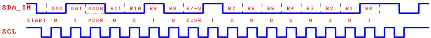
The figure above is a waveform diagram of the 12-bit data sent by the MCU to CH452 through a 2-line serial interface. The data is 001000000001B, and ADDR is used to select device addresses, which is represented by the dotted line in the figure.
