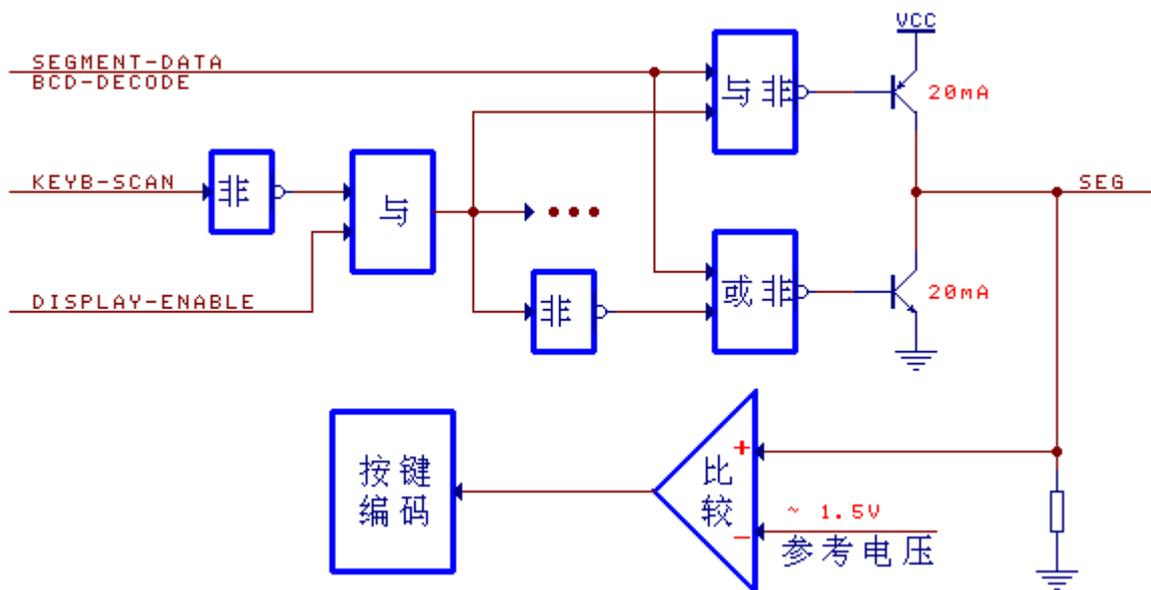
The following figure is the internal circuit diagram of CH452 word drive pins DIG7~DIG0.
